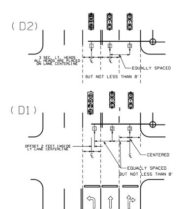
NOTE: WHERE LEFT TURN HEAD (HEAD 1 ON D1 AND D2) IS NOT CALLED FOR ON PLANS, MAST ARM LENGTH MAY STILL BE ALLOWED FOR FUTURE INSTALLATION. HEADS FOR THROUGH MOVEMENTS SHALL STILL BE ALIGNED WITH THROUGH LANES AS SHOWN ON DETAILS.
