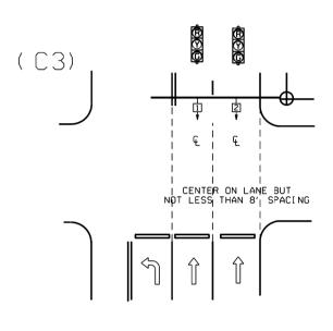
1. FOUR SECTION 'PROTECTED/PERMISSIVE' LEFT TURN HEADS SHOULD BE PLACED A MINIMUM OF TWO (2') FEET TO THE RIGHT OF THE CENTERLINE OF THE APPROACHING LEFT TURN LANE.
